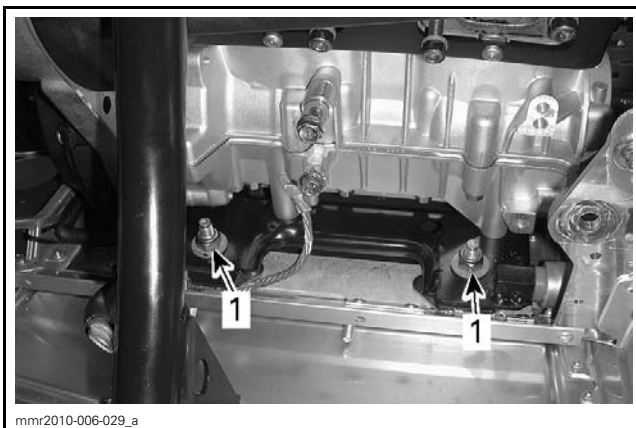
1. Front engine mounting nuts
