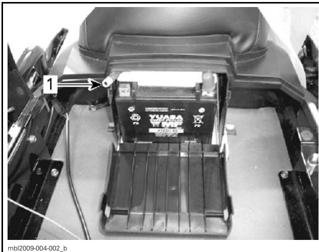
mbi2009-004-002_b INSIDE STORAGE COMPARTMENT 1. BLACK negative cable (-)
