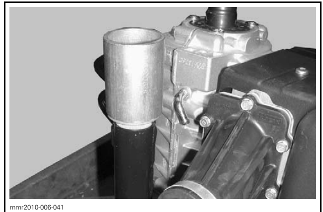
BALL JOINT INSTALLER OVER NEW ENGINE RUBBER MOUNT FOR INSTALLATION
